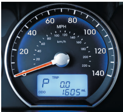
Figure 1.6 Many everyday items make use of both SI and British units. An example is this speedometer from a U.S.-built car, which shows the speed in both kilometers per hour (inner scale) and miles per hour (outer scale).
